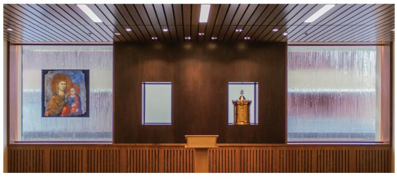
Texture: MD220 Atlas 3/8" Clear Tempered Kiln-Fired Glass 1-1/8" Insulated Units with 1/4" tempered PPG Solarban Z75
